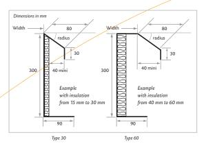
Sabliere in steel (2 mm thick) for renovation
